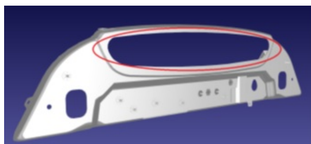
Figure 1. Rear firewall of a sports car to which a glass panel will be bonded. Example adhesive-application trajectory (red-line) that can be traveled with speeds based on the radius of curvature.
