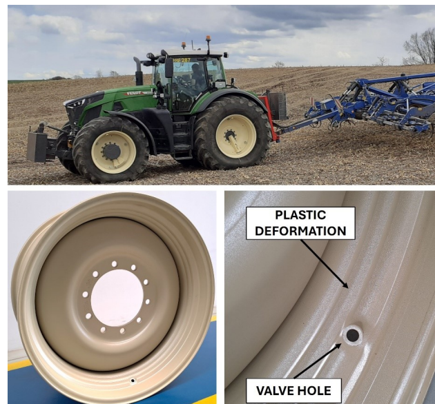
Figure 1. Example of an engineering application of the studied material. In agricultural wheels, the part of the wheel called rim is deformed plastically, and the tyre valve defines a dangerous notch which can reduce the material strength.
