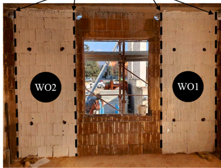
Fig. 2. Preparation of the one-way spanning walls (inside view).
