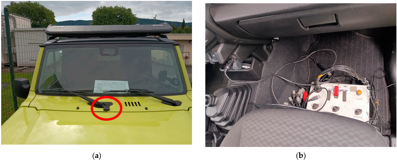
Figure 1. Location (a) of the GPS receiver (red circle), installed on the vehicle hood via magnetic connection, and (b) of the MoTeC ADL2 data acquisition unit, on the passenger mat, inside a protective box.
