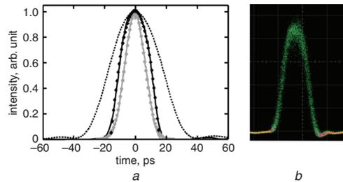
**Fig. 3** Temporal intensity profiles (Fig. 3a) of pump (dashed black line) compared with profile of idler wave obtained (after OBPF) for amplifier running in unsaturated and saturated regimes (solid grey and black lines, respectively). Full grey circles and full black diamonds represent a Gaussian and parabolic fits of temporal intensity profile, respectively. Oscilloscope trace in persistent mode of idler wave for amplifier running in saturated regime (Fig. 3b)
