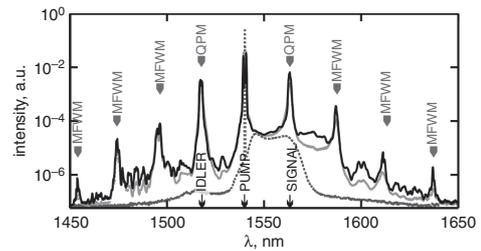
**Fig. 2** Optical spectra of pump wave (dotted dark grey line) compared with spectra at output of DOF with and without seeds (black and light grey solid line, respectively)
