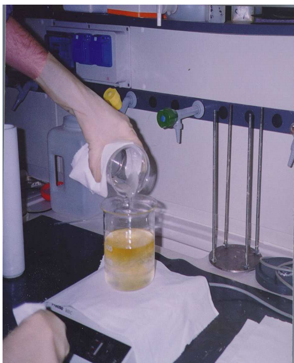
Figure 2.2: The decanting operation
