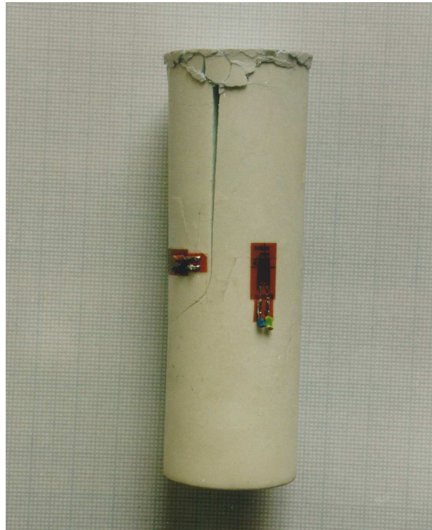
Figure 4.6: Compressive failure of a specimen made by syntactic foam type 1
