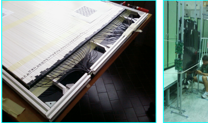
Figure 3.13: Photos of DANTE detector. Left, one of the 8 panel opened. In this photo the old configuration is shown, 30 bars through WLS to an adaptor for the MA-PMTs. A photo of the new configuration is shown in chapter 5. Right, photo of two panels forming a module ready to be setup in the experimental area.
