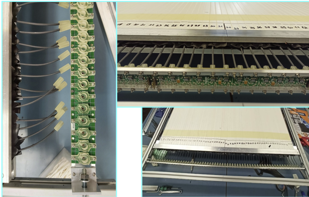
Figure 5.6: Photo of the final frontend configuration of a detector panel. On the left a photo showing the frontend board which hosts the SiPMs, the two part of the coupler 3d-printed, one attached to the SWL fiber the other screwed on the board. Top right the back detail of the structural support designed to hold the frontend board and to keep the bars aligned. Bottom right, photo of the whole frontend panel part without the panel enclosure.
