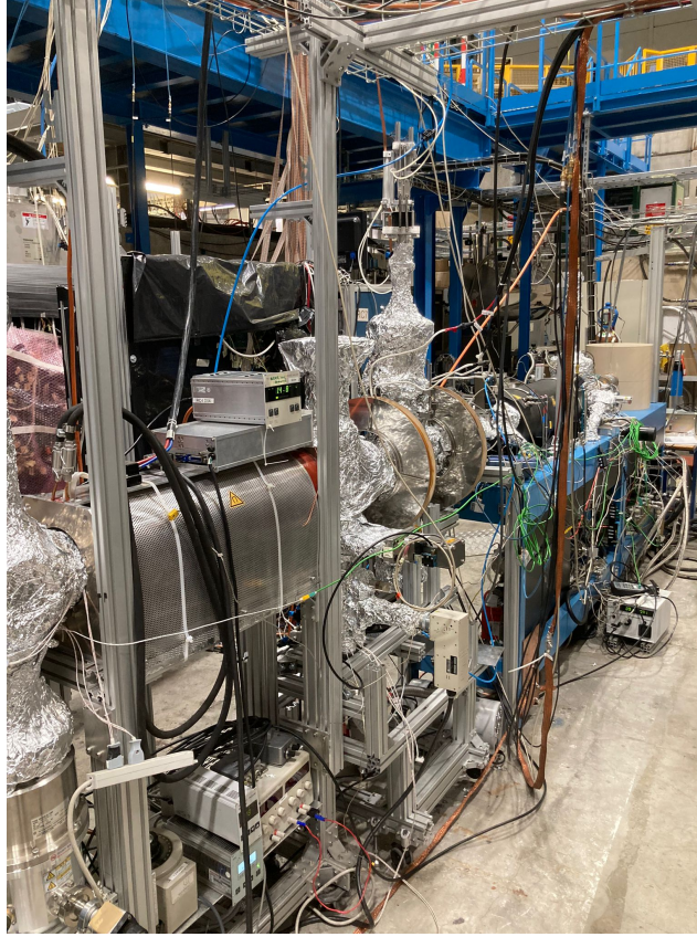
Figure 3.4: Photo of the positron apparatus. Shown from left to right are the STACKER, the FPS trap and the ^{22}\text{Na} source.
