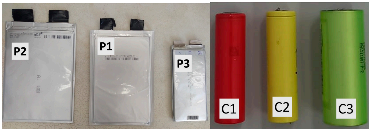
Figure 2. The three pouch type LIBs studied in this work (P1, P2, and P3), and the three cylindrical batteries found in the literature (C1, C2, and C3).
