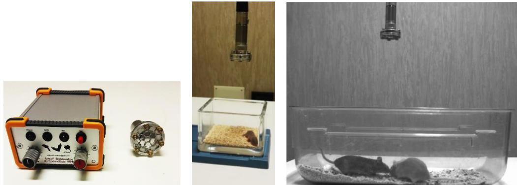
Figure 2. Mouse experimental settings to record USVs. Microphone (left panel) used to record calls during mother separation in pups (middle panel) and during adult male-female social interaction test (right panel).
