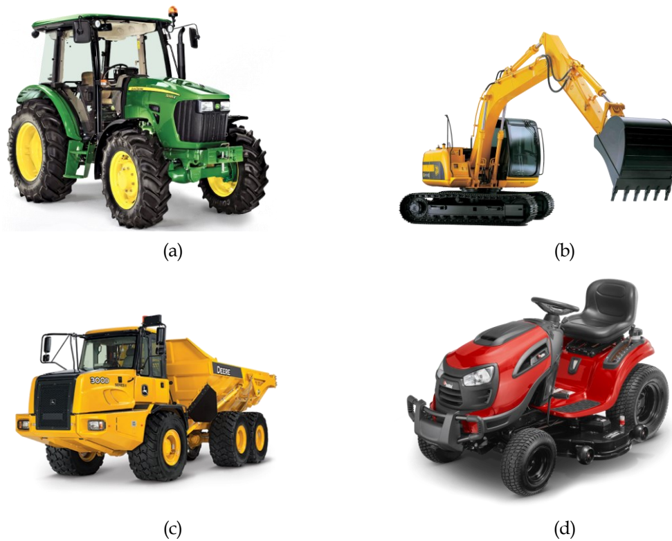
Figure 1.2 Examples of off-highway machinery. Agricultural tractor (a), excavator (b), mining dump truck (c), riding lawn mower (d).
