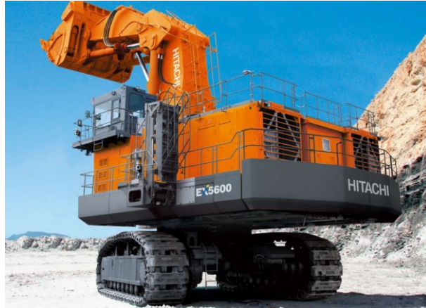
Figure 2.1 Example of tethered electric excavator, the Hitachi EX5600E.
