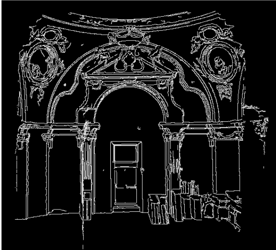
Figure 4. 3D edges extracted from reflectance image.
