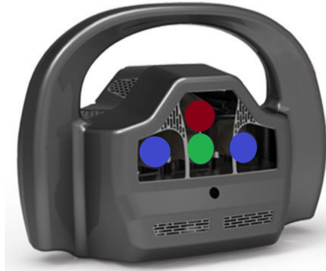
Figure 2.1: Render of the InSight scanner. Red dot: IR projector. Blue dots: IR cameras in stereo configuration. Green dot: color camera.
