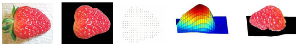
Figure 1.1: Example of shape from texture. From left to right: original image, segmented texture region, surface normals, depth map, reconstructed 3D shape. Image taken from [36]
