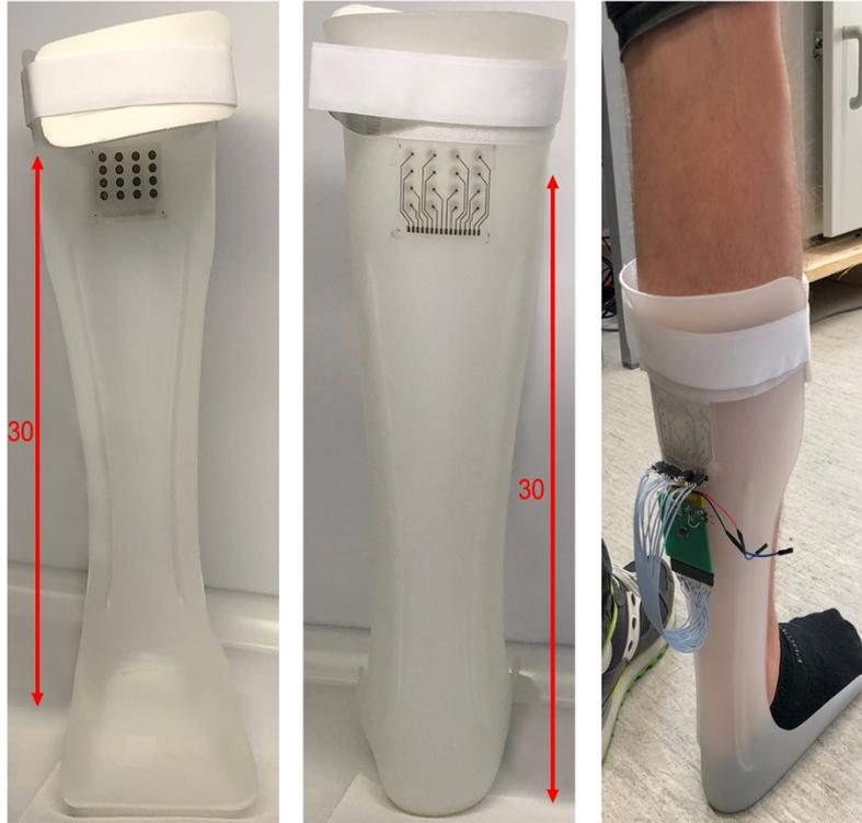
Fig. 12. Electrodes and tracks printed on the orthosis (quotes in cm); a tester wearing the devices with the electronics [66].
