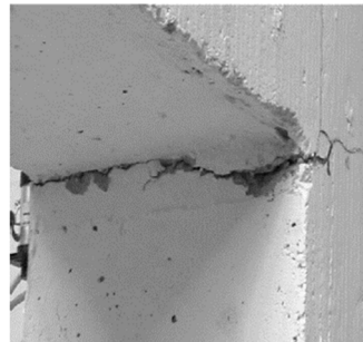
Figure 33: Experimental response of an internal 2:3 scaled joint: shear vs. top displacement curve a), sub-assembly crack pattern b) and focus on a beam-column interface. c) (Braga et al., 2009).
