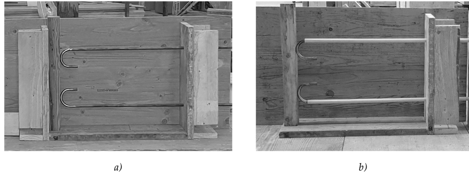
Figure 82: HS-type sample a) and H one with plastic pipe application b); pre-casting phase.
