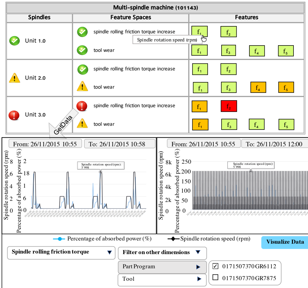
Figure 6.4: Visualisation of relevant data on operator's cockpit in the anomaly detection application scenario (GetData method).
