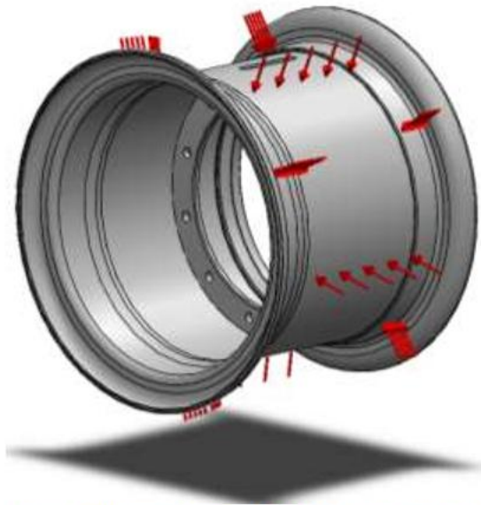
Figure 121 Pressure applied in the simulations on the lateral surfaces of the rim. The pressure is set equal to the inflation pressure.
