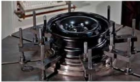
Figure 15 Machine for the rotating bending tests on rims. [13,14]
