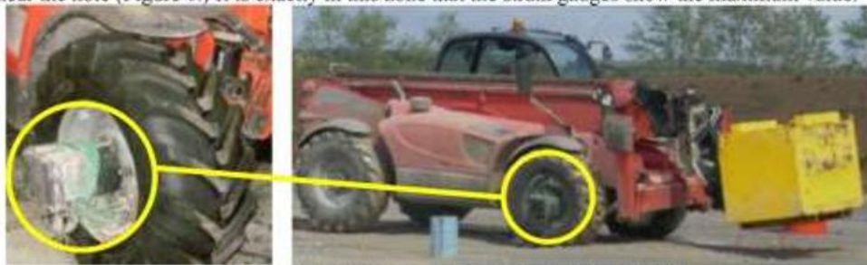
Figure 7 Position of a DAQ system on MANITOU TELEHANDLER
