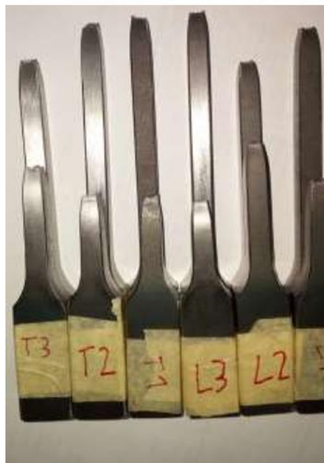
Figure 32 - Tensile test (3) - broken specimens
