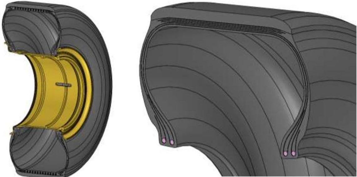
Figure 134 3D model of the tire to evaluate the loads exchanged between tire and rim.
