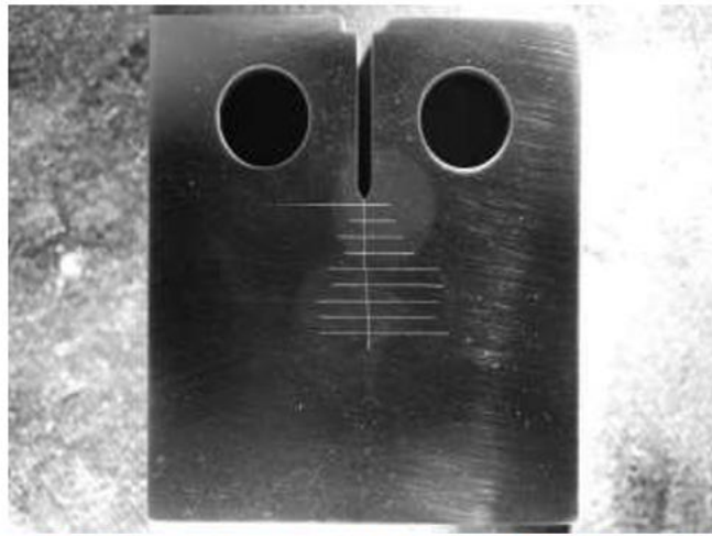
Figure 10 Notched specimen for fracture characterization of the material. On the specimen are clearly visible the crack occurred during the test and the measurements performed. [9]
