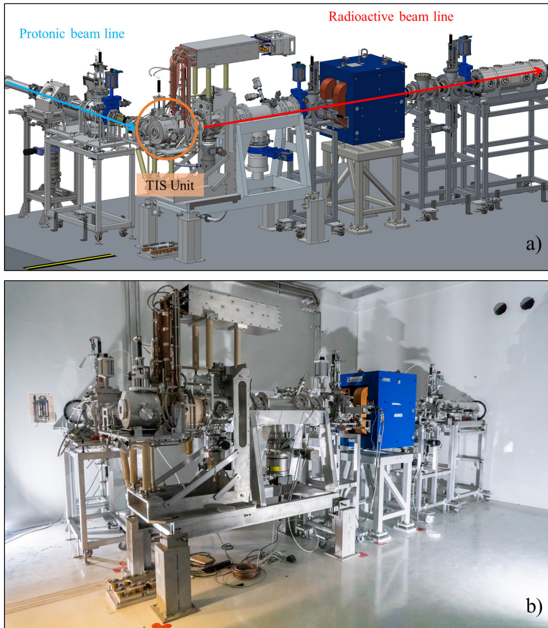
Figure 1.5 The CAD model (a) and a picture (b) of the Front-End installed inside the SPES bunker.
