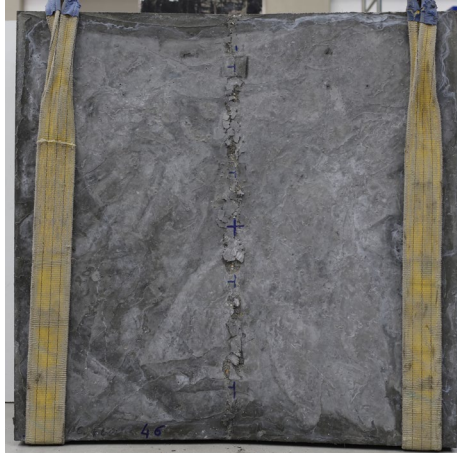
#12: P=106.2 kN, \tau=0.56 MPa, s=1.5 \mu\text{m} , w=14.2 mm
