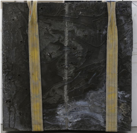
#11: P=95.9 kN, \tau=0.51 MPa, s=1.0 \mu\text{m} , w=10.1 mm
