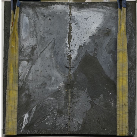
#5: P=94.3 kN, \tau=0.50 MPa, s=0.2 \mu\text{m} , w=15.1 mm
