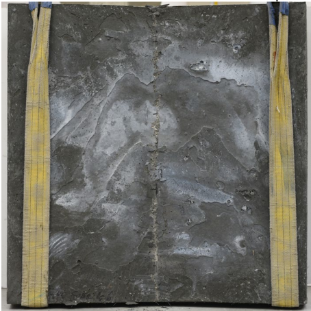
#4: P=96.8 kN, \tau=0.51 MPa, s=3.0 \mu\text{m} , w=17.0 mm
