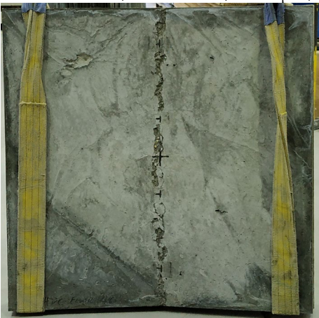
#10: P=90.1 kN, \tau=0.48 MPa, s=1.2 \mu\text{m} , w=12.8 mm
