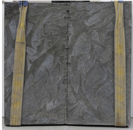
#1: P=105.8 kN, \tau=0.56 MPa, s=2.0 \mu\text{m} , w=11.9 mm
