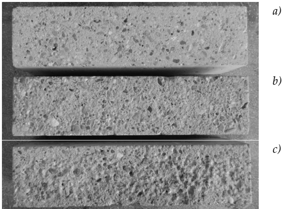
Figure 4.2-3: Comparison of the different substrate surfaces, a) smooth surface, b) rough surface and c) very rough surface.
