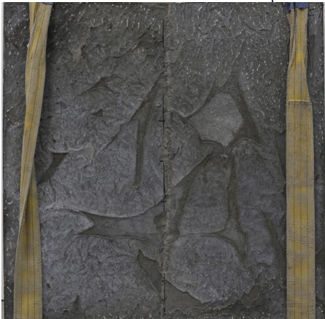
#4: P=102.5 kN, \tau=0.54 MPa, s=1.8 \mu\text{m} , w=13.1 mm
