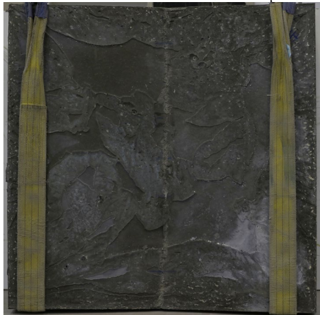
#7: P=96.2 kN, \tau=0.51 MPa, s=1.6 \mu\text{m} , w=10.6 mm
