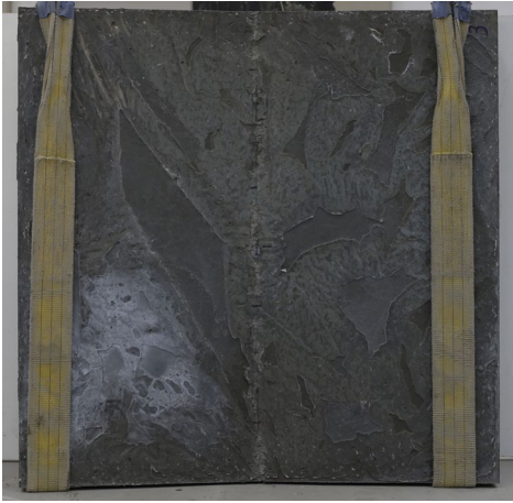
#3: P=93.6 kN, \tau=0.49 MPa, s=2.9 \mu\text{m} , w=15.4 mm
