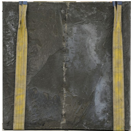
#1: P=110.6 kN, \tau=0.59 MPa, s=1.4 \mu\text{m} , w=12.9 mm
