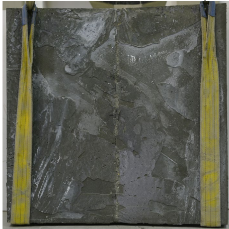
#7: P=91.6 kN, \tau=0.48 MPa, s=1.7 \mu\text{m} , w=13.3 mm
