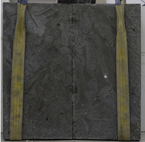
#10: P=100.5 kN, \tau=0.53 MPa, s=0.1 \mu\text{m} , w=11.6 mm
