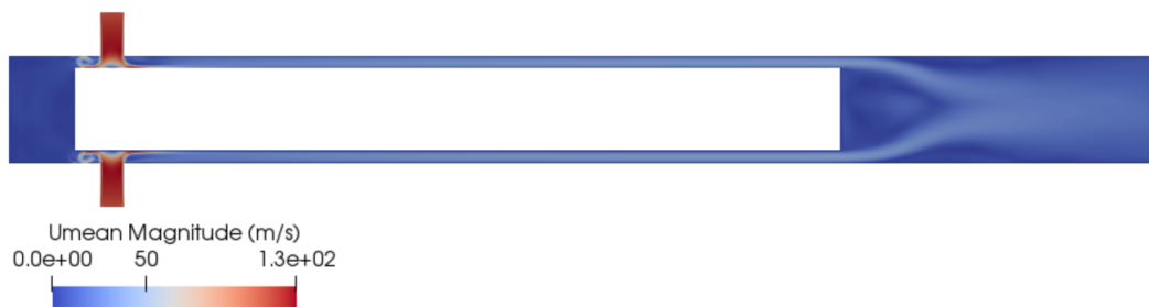
Fig. 3.18 LES computation: time-averaged velocity magnitude contours in the y-z plane
