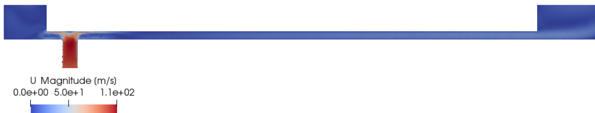
Fig. 2.9 Velocity magnitude field in the y - z plane - p_2 = 90 \text{ kPa} (Region close to the outlet not showed in the figure)
