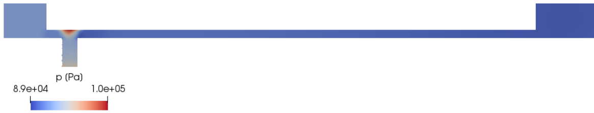
Fig. 2.10 Pressure field in the y - z plane - p_2 = 90 kPa (Region close to the outlet not showed in the figure)
