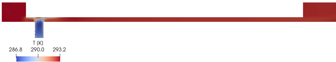
Fig. 2.11 Temperature field in the y - z plane - p_2 = 90 kPa (Region close to the outlet not showed in the figure)
