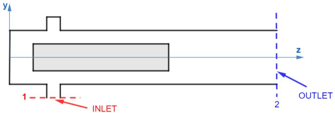
Fig. 2.8 Simplified gripper model for all CFD simulations
