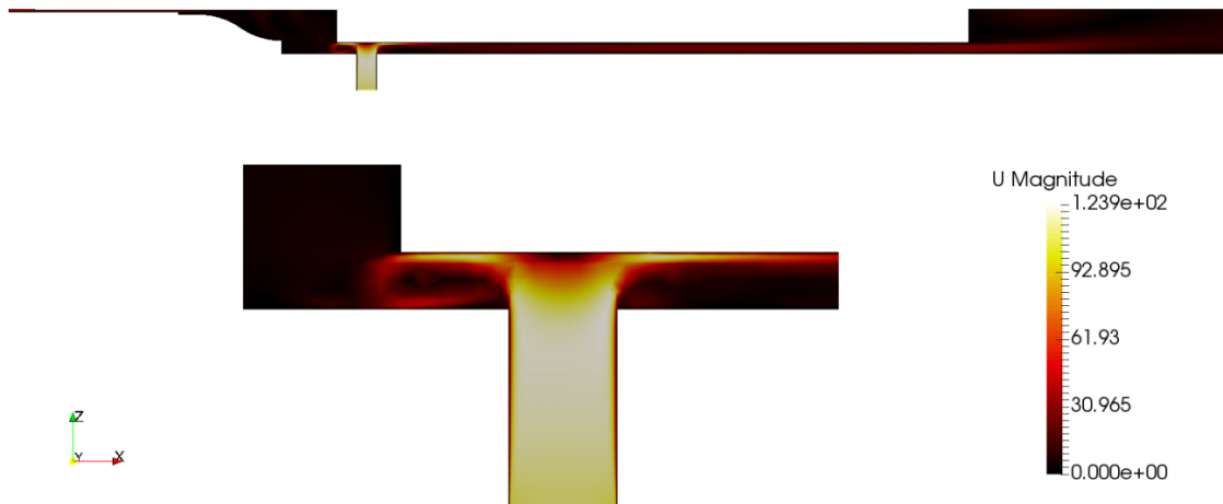
Fig. B.3 Velocity magnitude field at the middle plane - p_2 = 90 kPa
