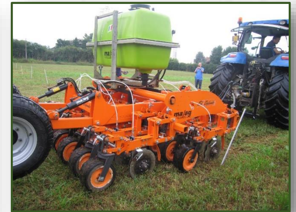
“Eco Defender 25” machinery for larval treatments with low impacts on soil structure
