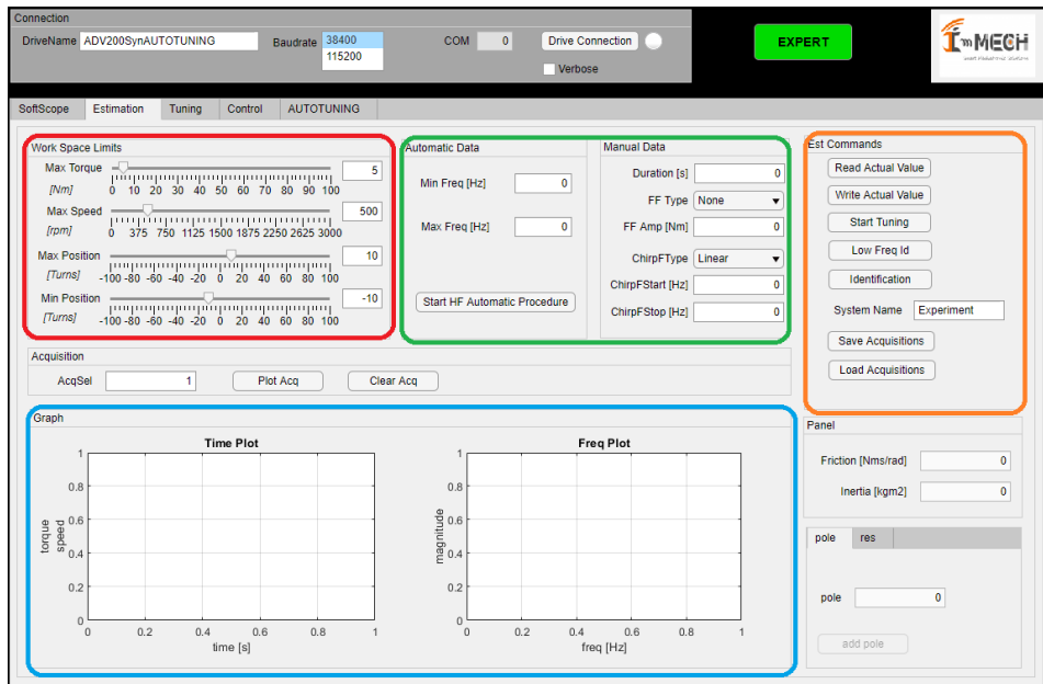
Figure 3.21: HMI for the application of the autotuning solutions, estimation window. The torque, velocity and position limits that must be respected during the excitation phase can be defined by changing the values inside the red box. The data for the excitation (e.g. max. and min. chirp frequencies) are defined by the values in the green box. The commands are given by means of the buttons inside the orange button, where it is possible to launch different identification procedures (e.g. low frequencies identification, full-range frequencies identification). The results are then shown in the graphs of the blue box.
