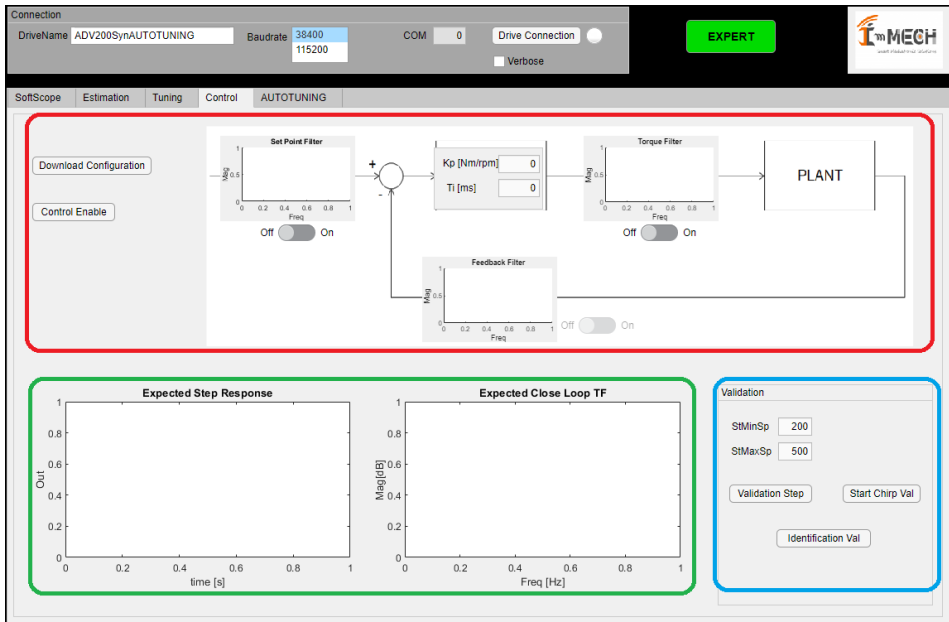
Figure 3.23: Validation interface. The tuned control is graphically shown in the scheme inside the red box, where the various filters can be switched on and off. The validation tests can be launched acting on the buttons inside the blue box, and the resulting performance can be compared to the expected ones by checking the graphs inside the green box.
