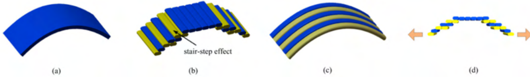
Figure 1.23: Comparison between the surface quality (a and b) and the mechanical strength (c and d) of CLFD (left) and flat FDM (right) [38].
