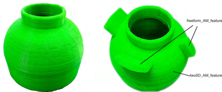
Figure 1.6: The fins added to the jar are an example of free-form AM features [6].
