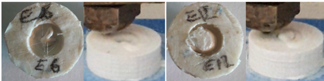
Figure 6.7: New layer: two case with under-extrusion (6mm and 12mm) to witness the anchor formation
