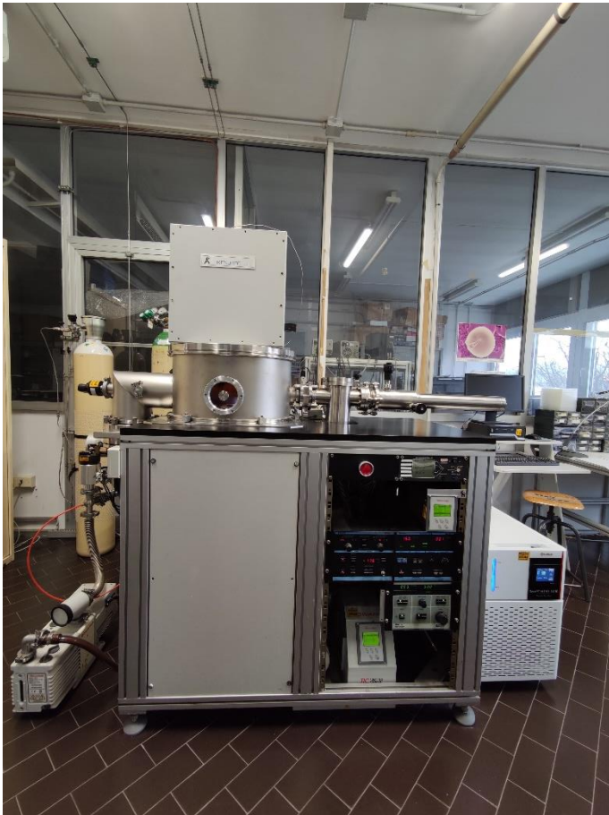
Figure 15. Magnetron sputtering system.
