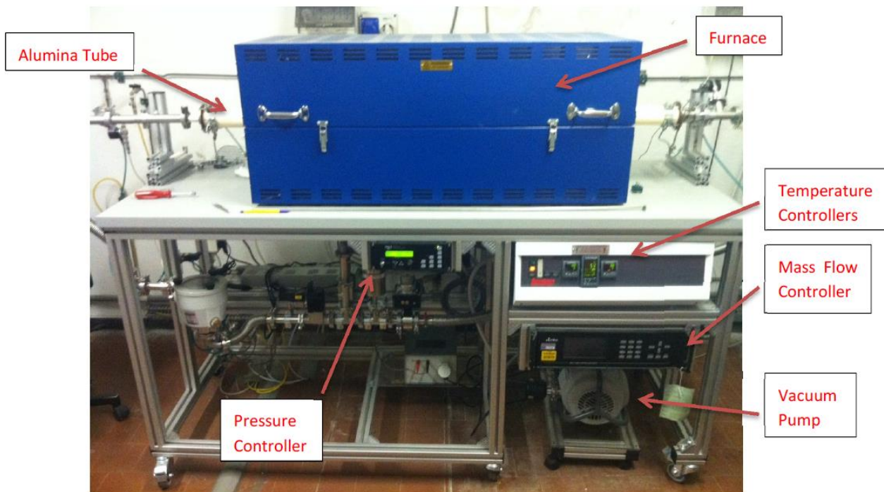
Figure 16. Vapor-phase growth custom furnace
