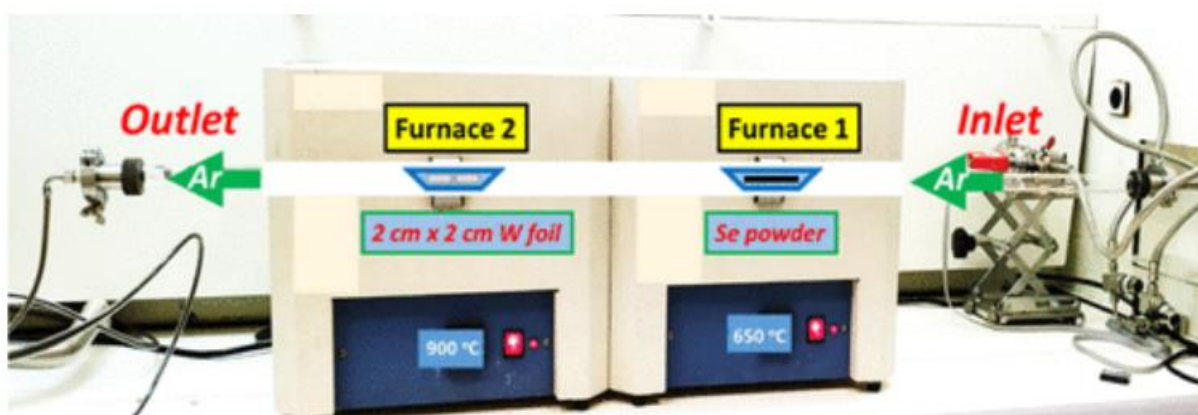
Figure 18. APCVD experimental setup.
