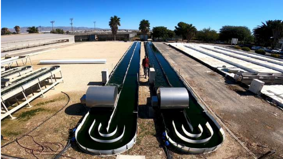
Figure 2.1: Raceway reactors located at IFAPA research center.
