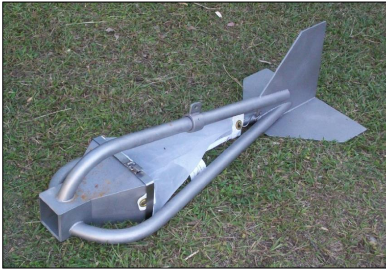
Figure 3.10 – The Helley-Smith bedload sampler [Erskine et al., 2011]
