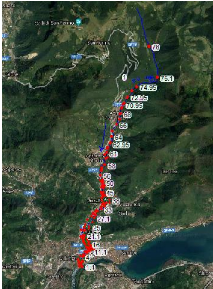
Figure 5.56 – Guerna creek in the HEC-RAS model
