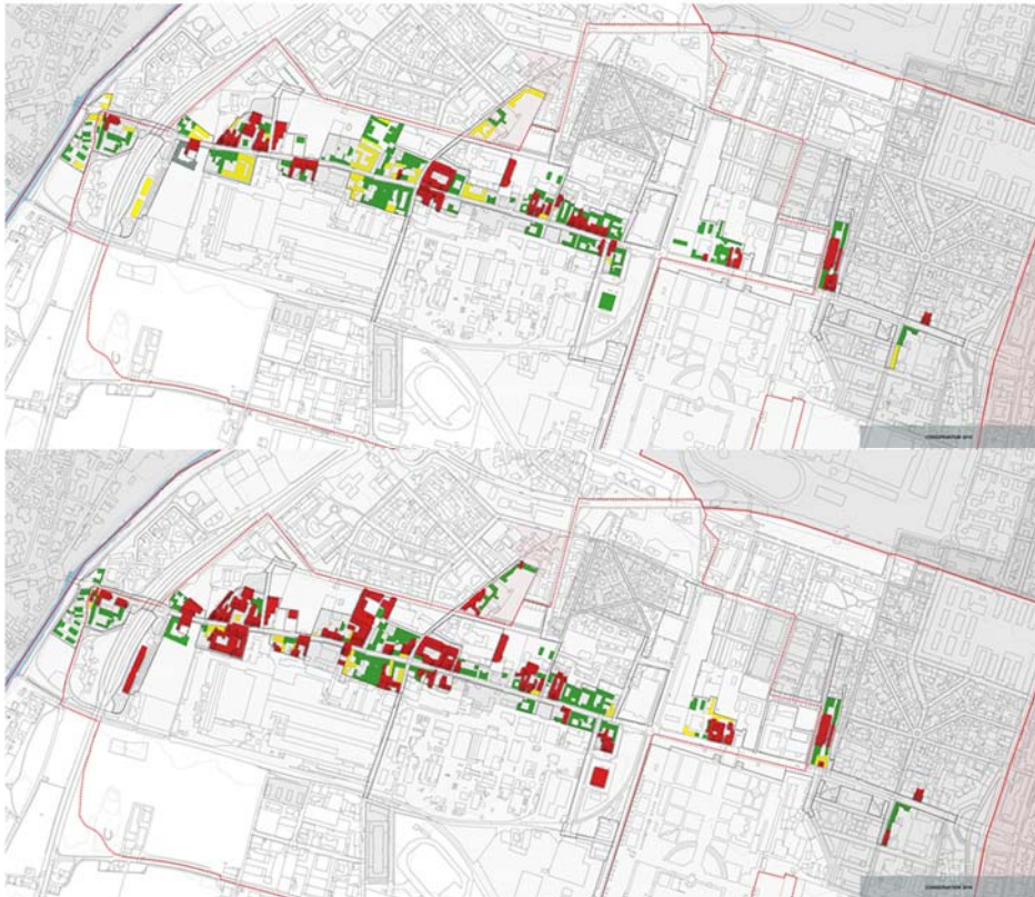
Fig.3 The conservation state of buildings in 2010 (up) and in 2018 (down); the red-3D buildings are the ones in a worst state of conservation, the yellow buildings are the partially deteriorated and the green ones represent buildings in a good state of conservation. It is possible to see that the red buildings are increased.
