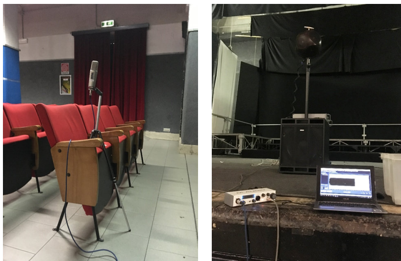
Figure 1: Experimental setup: microphone (left); source and acquisition equipment (right).
