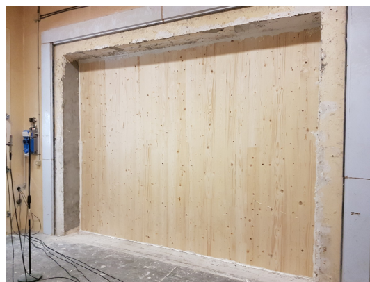
Figure 2: CLT panel undergoing tests in sound transmission suites.
