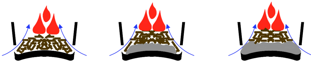
Figure 5: Sketch of combustion evolution in the new type of burning pot (stoves B1 and B2)
