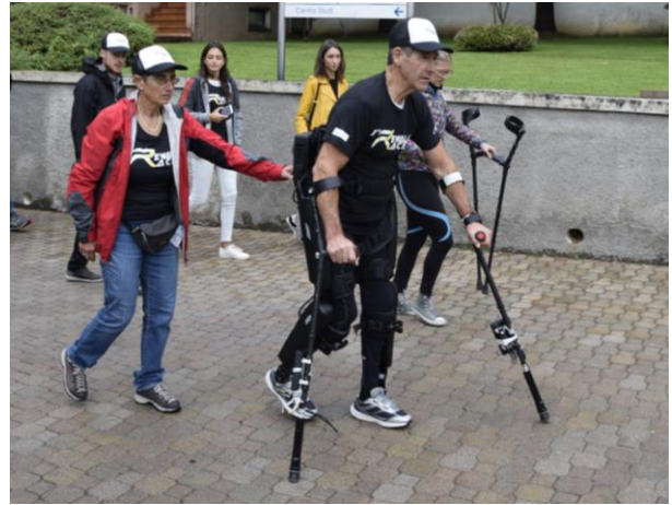
Fig. 1. An expert user of a Rewalk P5 device, while practicing with the exoskeleton and the instrumented crutches presented in this work.
