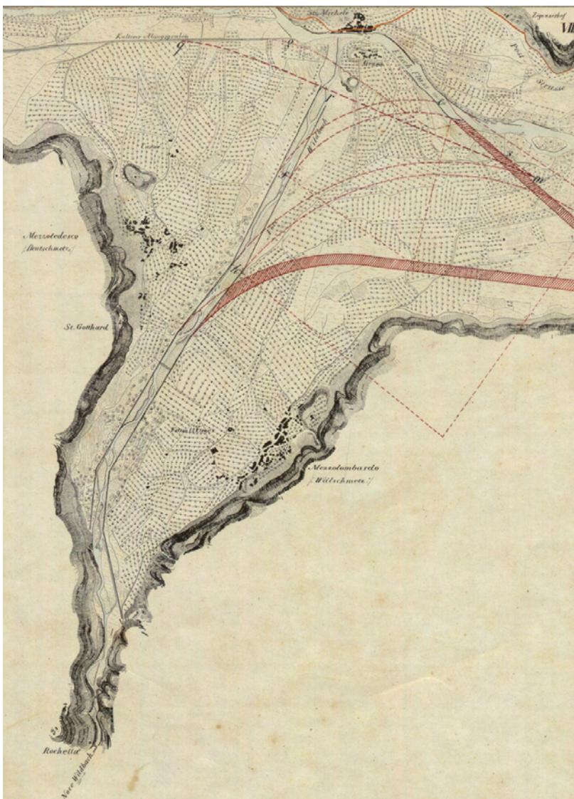
Figure 2. A detail of the Claricini “Tridentina” map sheet nr. VIII at the junction of the Noce with the Adige River. Three hypotheses of the Noce river diversion, completed in the year 1853, are sketched. It is worth noticing the Italian and German names of the towns of Mezzotedesco/Deutschmetz and Mezzolombardo/Wälschmetz, the only bilingual toponyms on the 14 map sheets. (©courtesy of TEMI Editrice, Trento)
