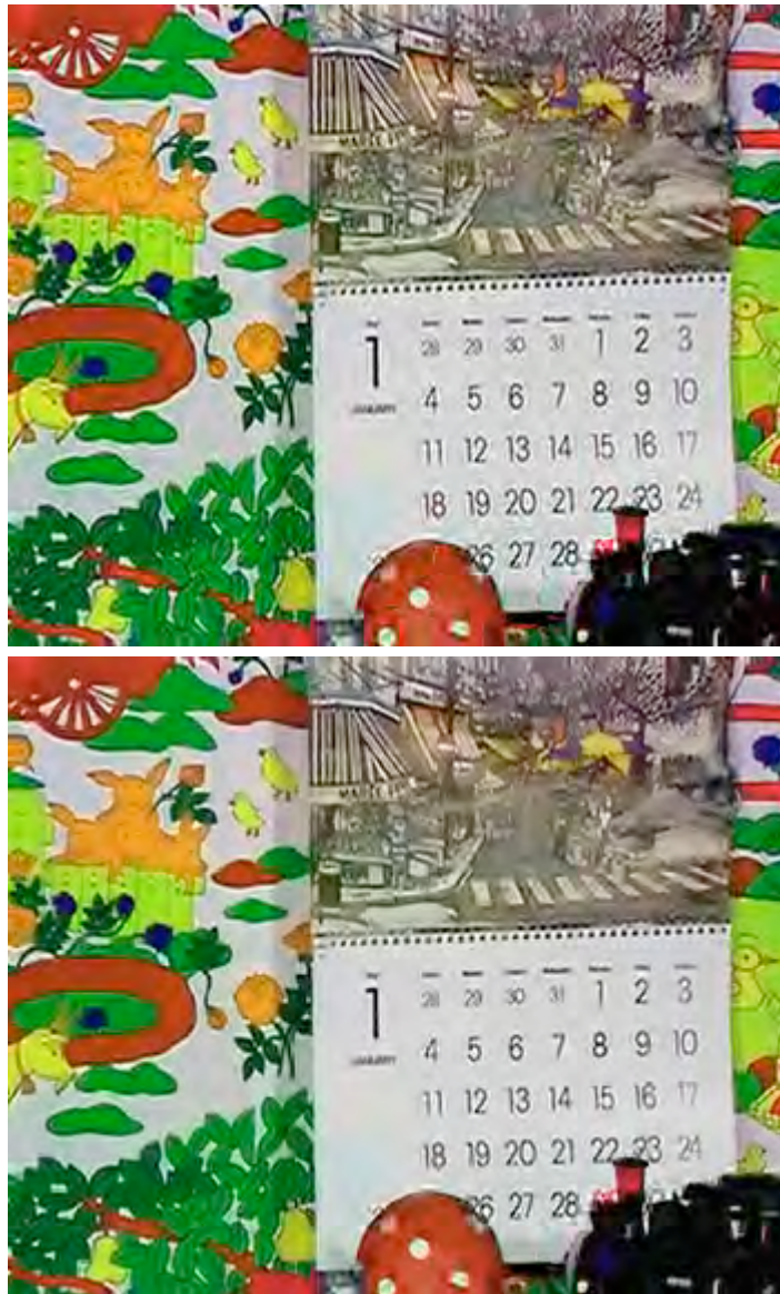
Figure 18 (a)-(c) Visual results with (bottom) and without (top) the use of the de-ringing filter
