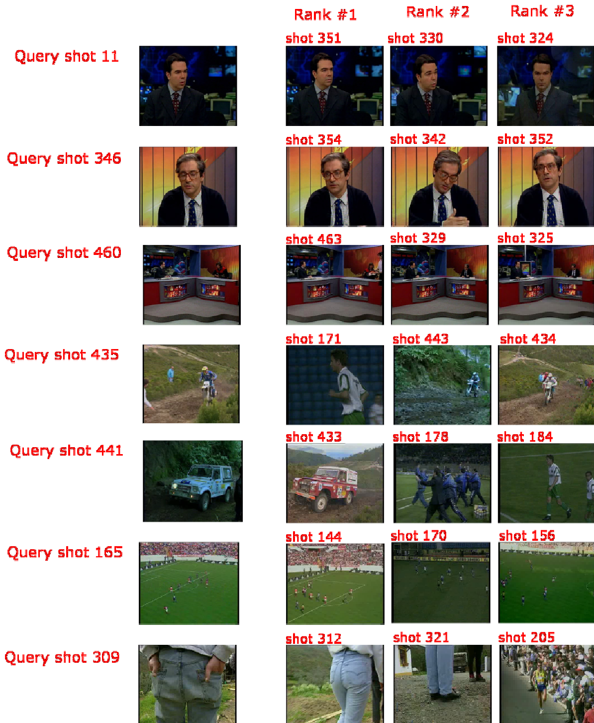
Figure 6: Examples of motion-based shot retrieval: ‘low’ activity scenes (query shot 11, 346, 460) - anchorperson, interviews; ‘high’ activity shots (query shot 435, 441, 165, 309) - motor biking, motor racing, football matches, close-up motions. The retrieved shots on the right exhibit similar motion characteristics to those of the query shots, respectively, even though they may show different visual contents.
