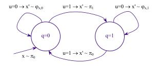
Fig. 1. Controlled Markov chain model.
