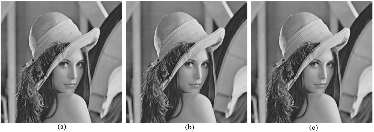
Figure 5. Coding results for Lena. (a) Original image. (b) Compressed image at 0.5 bpp. (c) Compressed image at 0.25 bpp.
