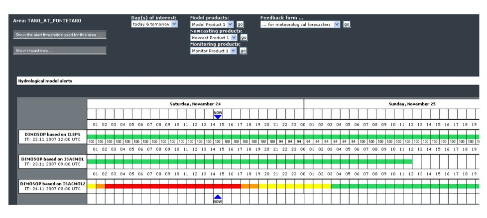
A visualization of the operational flood forecasting chains for the Taro River during the MAP D-Phase experiment. Different colours refer to different alert levels: no alert (green), alert for an event with a return period of at least 60 days (yellow), of at least 180 days (orange) or of at least 10 years (red).
