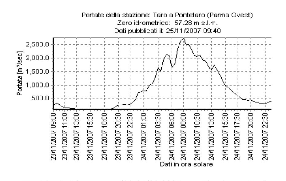
The Map D-Phase event (21-25/11/2007- see Fig. 6) provided a peak discharge value of 2696 m3/s, corresponding to a specific discharge of about 1.8 m3/s/km2. The peak discharge was recorded at 7:00 UTC of the 24th November.
