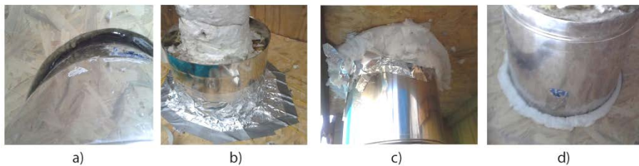
Figure 3. Tested clearance sealing mode: a) open ( op ), b) sealed with metal sheet ( ms ), c) sealed with insulating material ( ad ), d) filled with insulating material ( fi ).
