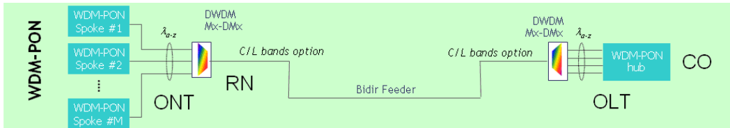
Figure 1. Self-seeding based architecture.
