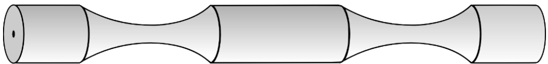
Figure 4. Schematic representation of a bi-taper in optical fiber, very common configuration for a Mach-Zehnder interferometer.
