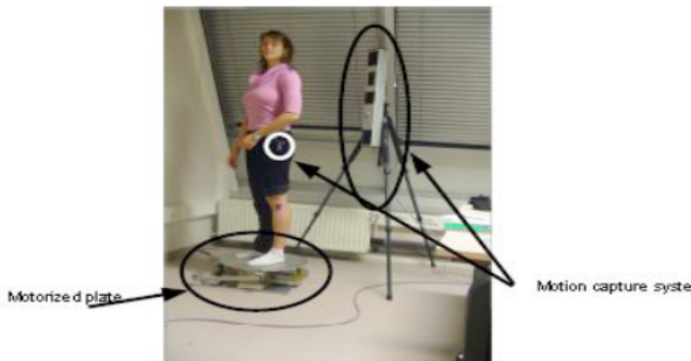
Fig. 4: Dynamic platform for postural disturbance. The Italian student Fabio Spazzini has developed the control of this device enslaving its motion to a motion capture system at UPMC as project for his Master degree.
