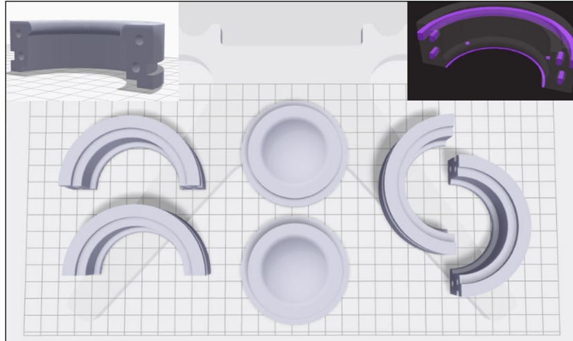
Figure 5 – Printing plate composed by two replica of the polymer dies with a 3D detail on the support material filling (in purple).
