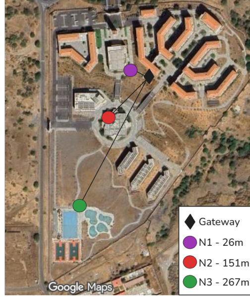
Figure 2.10: Geographical deployment of the three sensor nodes and the gateway at the field site in Praia, Cabo Verde.
