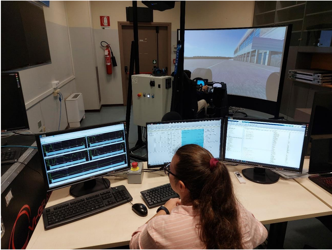
Figure 3.24. PC station of the compact driving simulator: for data analysis during tests, for setting the simulation environment and for saving test data.
