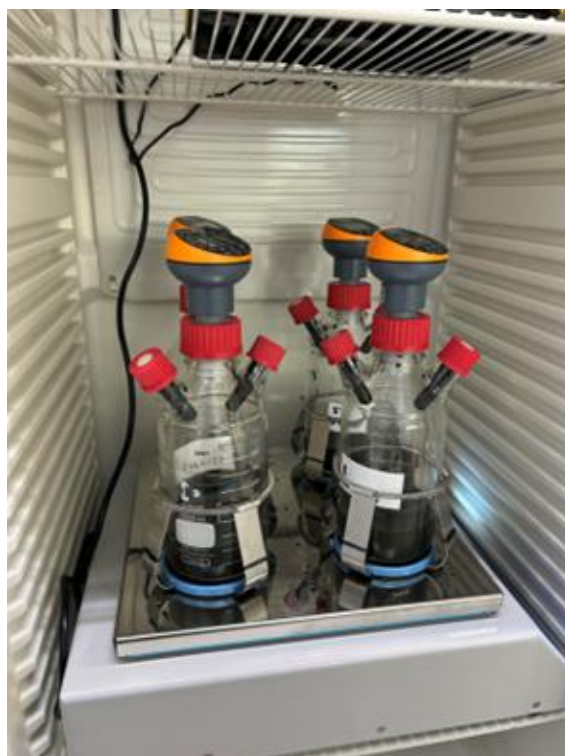
Fig. 6.1. A) Schematic of the fermentation experiment. B) Co-digestion of FJPWW and PS BMP test using the OxiTop®-IDS AN 6 system.
