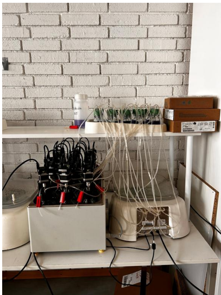
Fig. E.6. SMA of granules from R2S reactors treating FJPWW using the AMPTS II® system.
