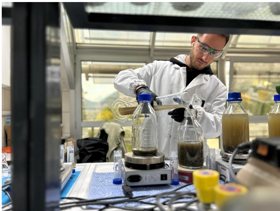
Fig. E.5. FJPWW and PS co-fermentation test preparation.
