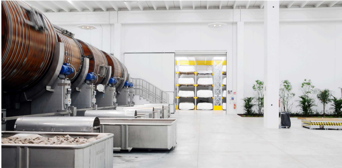
Figure 2 - Wet-end processing department of a tannery
