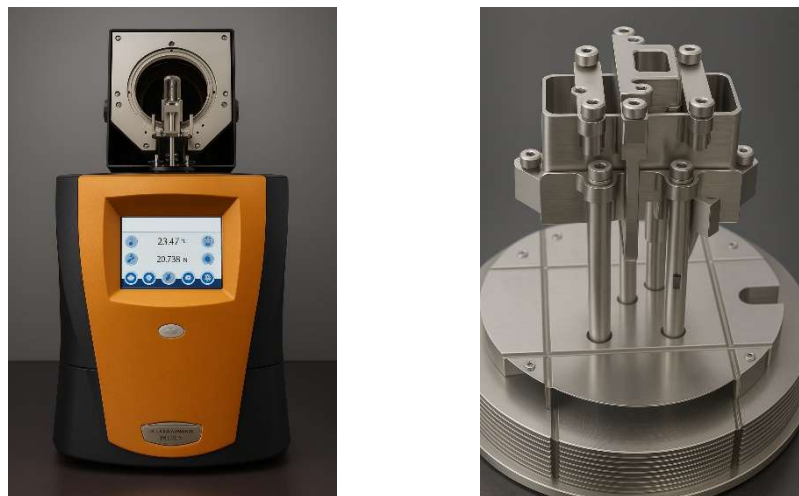
Figure 13 - DMA 850 of TA instrument that is equipped with a submersion film clamp
