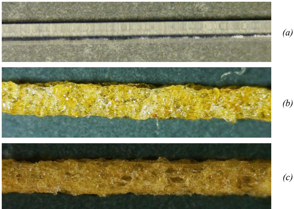
Figure 42 - Details of paths printed at 50 mm/s for (a) TPU at 220 °C, (b) 20 wt % and (c) 30 wt % at 225 °C
