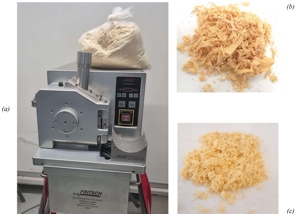
Figure 21 - Grinder (a), glutaraldehyde shavings (b) and ground leather particles (c)
