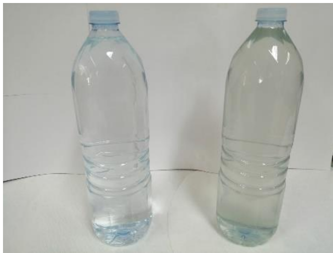
Figure G. 21 Raw greywater(right) and Treated graywater (left)
