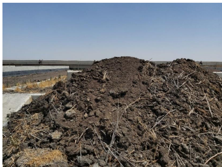
Figure A. 15 Dry sludge – Mafraq WWTP
