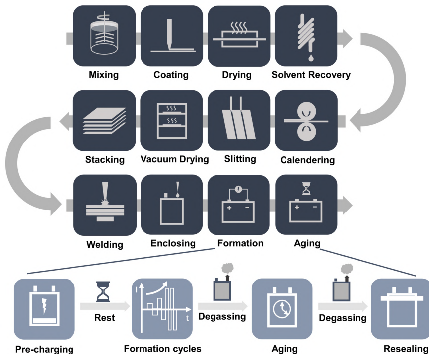
Figure 2.7: Schematic representation of lithium ion battery fabrication process [213].
