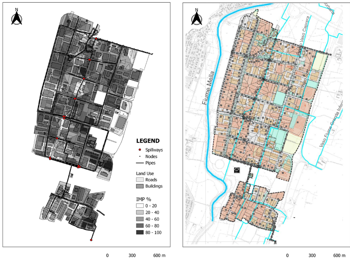
Fig. 46 – a) Generalized map of the study area with subcatchments and sewerage network, b) SWMM Model with background.
