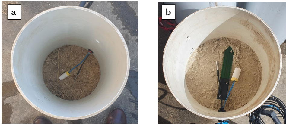
Fig. 14 – a) Lower sensor cluster comprised of 1 Chameleon Soil Water Sensor and 1 DS180B20 digital temperature probe, b) Upper sensor cluster comprised of 1 Chameleon Soil Water Sensor, 1 DS180B20 digital temperature probe and 1 Truebner SMT 100 soil moisture and temperature probe (Photo by Leigh Oliver)
