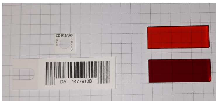
Figure 1.7: RCF films (on the left) and radiochromic PMMA dosimeters (on the right). Squares in the background are 5 x 5 mm.
