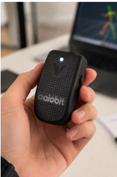
Figure 1. Wearable IMU sensor implemented in the study for trunk motion analysis
