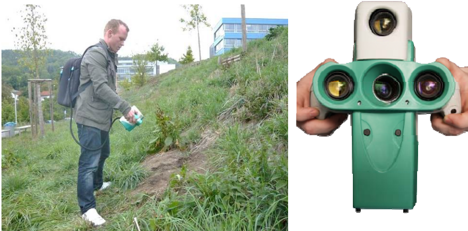
Fig. 2: Handheld 3D-Scanner “kolibri Cordless” for outdoor data capturing
